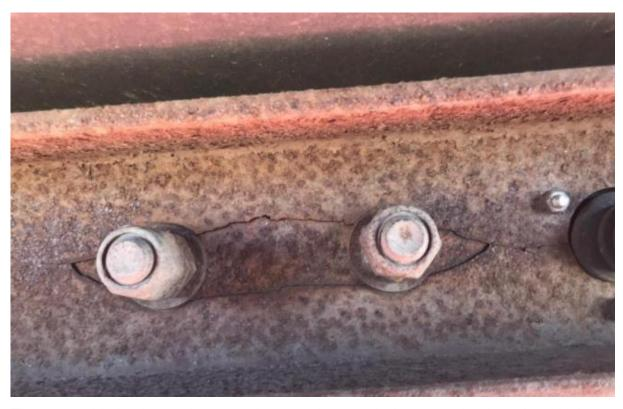
The nuts and bolts shown above are those used to attach the towing hook to the vehicle.
