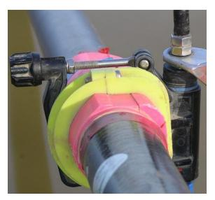
Incorrectly closed (the nut at the end of the top bar is not tightly closed against the cylindrical collar that surrounds the top bar).
