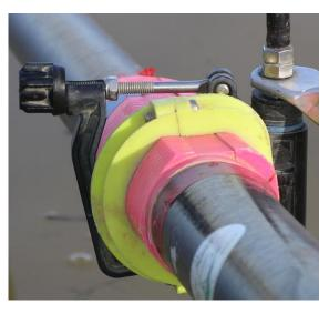
Incorrectly closed (the nut at the end of the top bar is tightly closed against the end of the cylindrical collar that surrounds the top bar but the cylindrical collar is not fitted into the groove in the nut).
